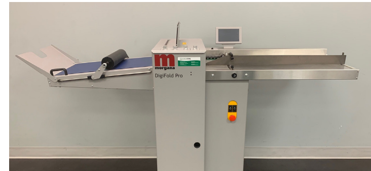
Morgana Digifold Pro Creaser/Folder Was: $22,995 NOW: $19,995 Crease and fold up to 6000sph/400gsm; 7" SmartScreen and memory to store common jobs.
