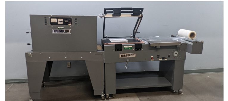
Beseler T-18-8 Shrinkwrapping System Was: $8,495 NOW: $6,495 18"W x 8"H x 36" L tunnel chamber w/adjustable air dampers & automatic cool down
