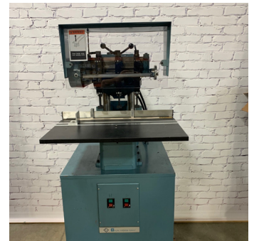
Baum K3 Hydraulic 3-Head Drill Was: $3,500 NOW: $2,995 3-spindle drill with side guides
