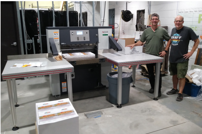
Printhub.ink's new Mohr D80 ECO hydraulic cutter including side air tables.
