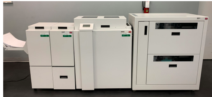
Morgana AF 2000S Bookletmaker Was $39,995 NOW: $37,495 AF 602 set feeder with two high pile bins; BM 2000S bookletmaker includes 2x ISP heads with inline face trimming and squareback unit; Fully automatic bookletmaking with 30 sheet capacity
