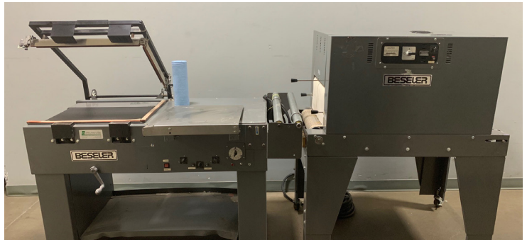
Beseler T-18-8 Shrinkwrapper Was: $8,995 NOW: $8,495 18" wide, 8" tall and 36" long tunnel chamber w/ adjustable air dampers & auto cool down
