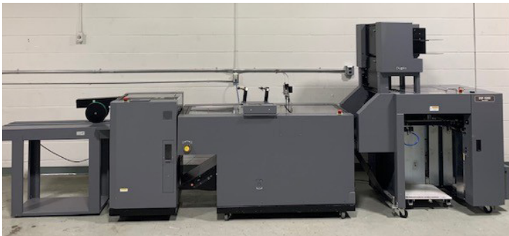
DSF 5000 High-Capacity Booklet System Configured w/ DSF 5000 set feeder w/optional cover feeder, SCC side slit/crease module, DBM 500 Bookletmaker w/optional spine flattener & 500T face trimmer. Please call to discuss configuration requirements and price.
