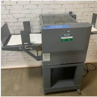
Duplo DC-445 w/ Perf Attachment Was: $8,995 NOW: $8,495 Air suction feed; up to 15 creases, 3000sph
