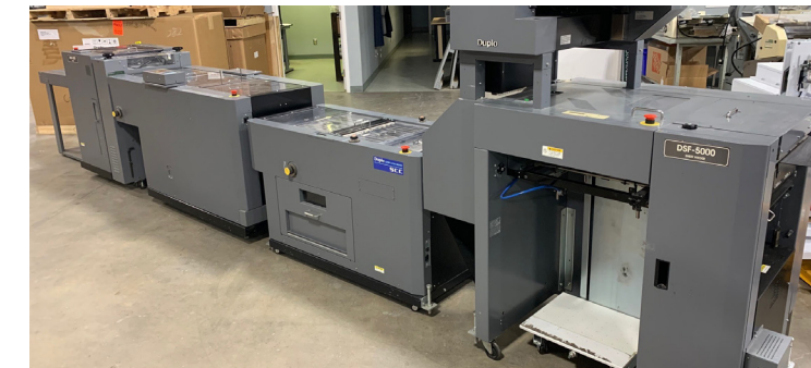
DSF 5000 High-Capacity Digital Bookletmaker System Configured w/ DSF 5000 set feeder w/optional cover feeder, SCC side slit/crease module, DBM 500 Bookletmaker w/optional spine flattener & 500T face trimmer. Please call to discuss configuration requirements and price.
