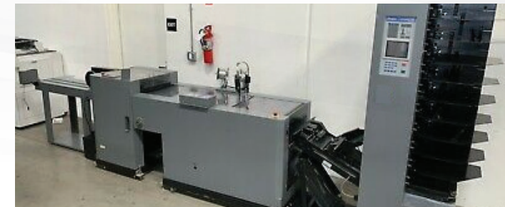
DUPLO 5000 SINGLE TOWER SYSTEM BOOKLET-MAKING SYSTEM 14 x 20 MAX SHEET WITH FULLY AUTOMATIC SETUP
